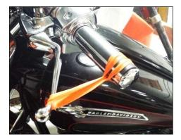
e) While still in **NEUTRAL**, quickly rev the engine between 3,000-5,000 RPM (1/4 to 1/2 throttle), then let it return to idle. Notice the movement in the clutch lever when the engine is revved. This is your Free Play Gain.
