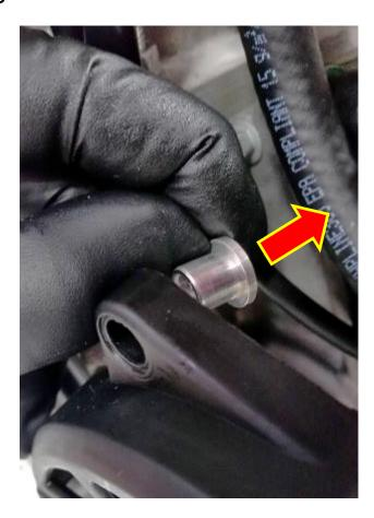
9. Insert the new provided chain guard screw sleeve into the screw slot, then reattach the chain guard to the slave cylinder using the longer OE screw.
