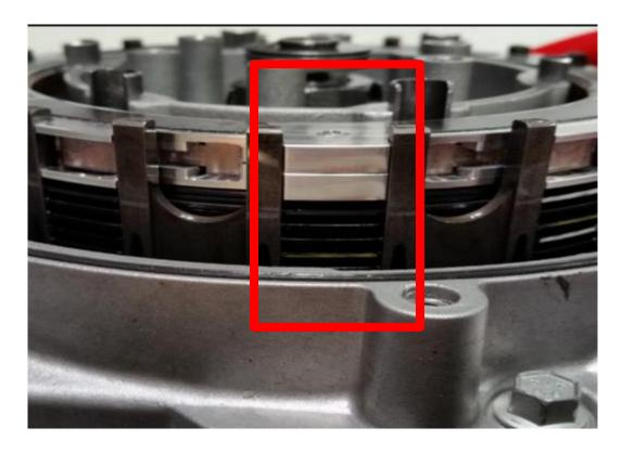
1. Soak the EXP disk and friction disks in new engine oil for 5 minutes. Make sure the EXP and friction disks are coated in oil on both sides.
