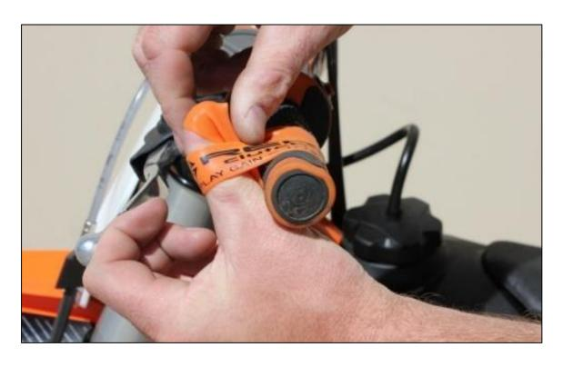
d) Pull the band through the loop, then attach it to the outside end of the clutch lever. This will take up the initial free play (slack) and put the lever in a position to detect the Free Play Gain.
