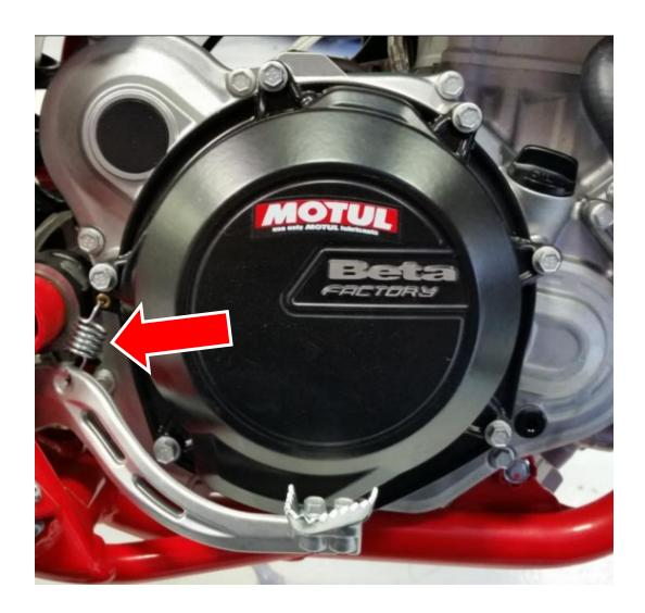
5. Using an 8 mm socket, remove the OE clutch cover. Pay close attention to the length and location of the OE screws so they can be returned to their same location.
