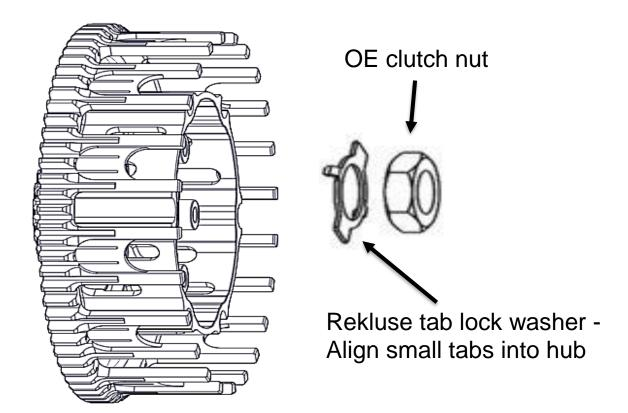
4. Using the socket and torque wrench, torque the center clutch nut to **50** ft-lb (**68** N-m).
