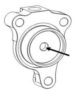
3. Pour the manufacturer recommended clutch fluid into the slave cylinder port.
