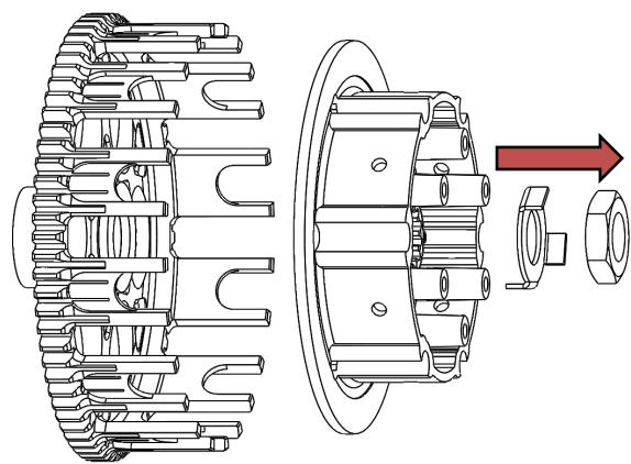
**Note:** Check that the OE thrust washer is still on the main shaft and not stuck to the bottom of the center hub assembly. The thrust washer must be installed or clutch performance issues will result.
