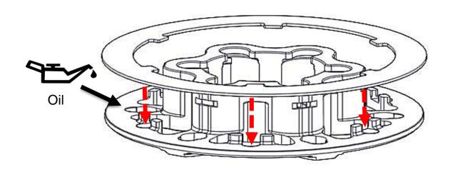
6. Install the Rekluse pressure plate, pressure plate springs, screw sleeves, and pressure plate bolts.
