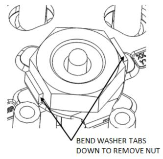
12. Remove the center clutch nut with an impact wrench or breaker bar, and socket. Set aside. The OE clutch nut will be reused.
