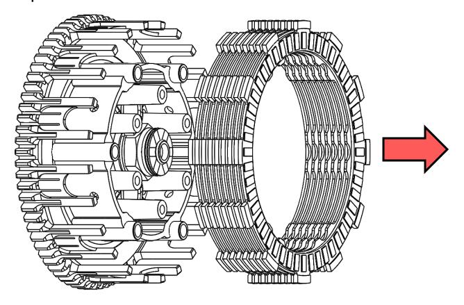
8. Remove the 6 drive pins. Set these aside. The drive pins will be reused.
