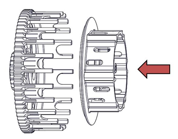
2. Install the new Rekluse tab washer with the bent tabs facing down, aligning with the holes in the hub.
