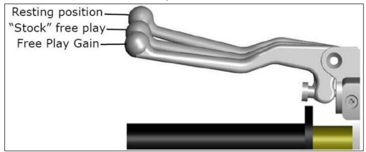
If there is too much Free Play Gain, the installed gap is too small. The bike may drag and stall because it has difficulty disengaging the clutch. It may also be difficult to shift. Too much Free Play Gain will not hurt the clutch, but it will negatively affect clutch performance.
