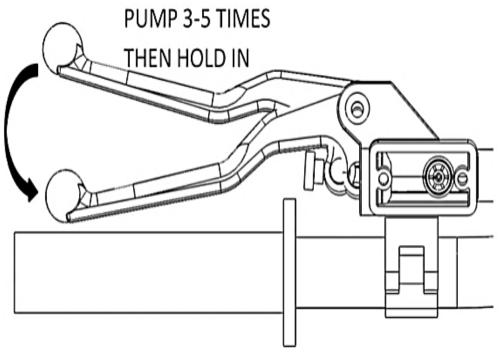
5. While still holding the clutch lever in, use a wrench to open the bleed port. Air and fluid should flow from the bleed tube.
