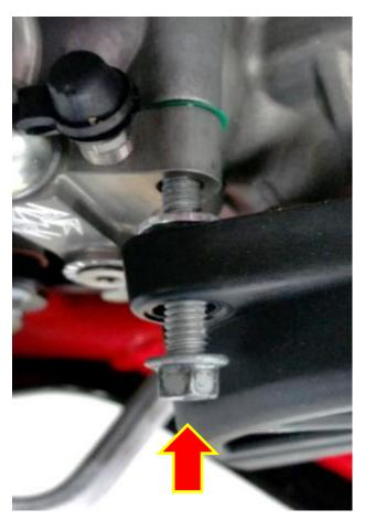
**Note:** The Rekluse screw sleeve is slightly taller than the OE screw sleeve. You will need to use the Rekluse screw sleeve to help ensure a good seal to the engine case.
