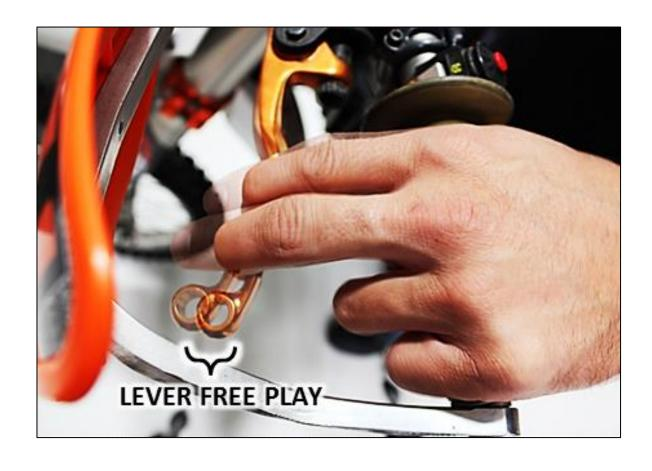
c) While still in **NEUTRAL**, continue to apply light pressure and quickly rev the engine between 5,000-7,000 RPM (1/2 to ¾ throttle), then let it return to idle. Notice the movement in the clutch lever when the engine is revved. This is your Free Play Gain.
