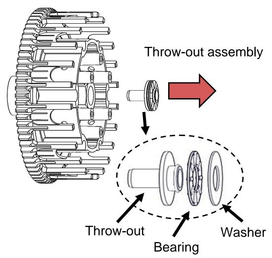
11. Use a hammer and large screwdriver to bend down the edges of the washer tab until it clears the clutch nut.
