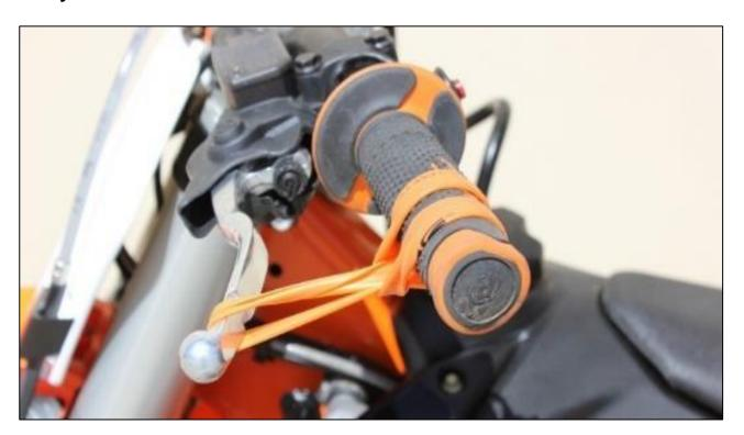
e) While still in **NEUTRAL**, quickly rev the engine between 5,000-7,000 RPM (1/2 to ¾ throttle), then let it return to idle. Notice the movement in the clutch lever when the engine is revved. This is your Free Play Gain.
