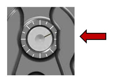
Use the tick marks on the cylinder and the etch mark on the screw to remember the starting point for adjusting the gap.
