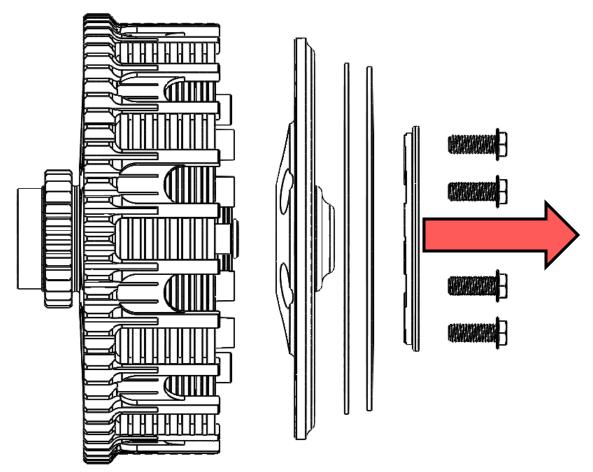
7. Remove the OE clutch pack, then set it aside. The pack will not be reused. Use a pick if necessary to help remove the clutch pack.
