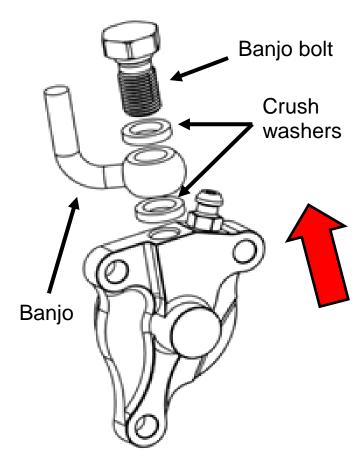
4. Attach the clutch fluid line to the Rekluse slave cylinder using the OE banjo bolt and the 2 new crush washers from Rekluse. Make sure the banjo is sandwiched between the 2 crush washers.
