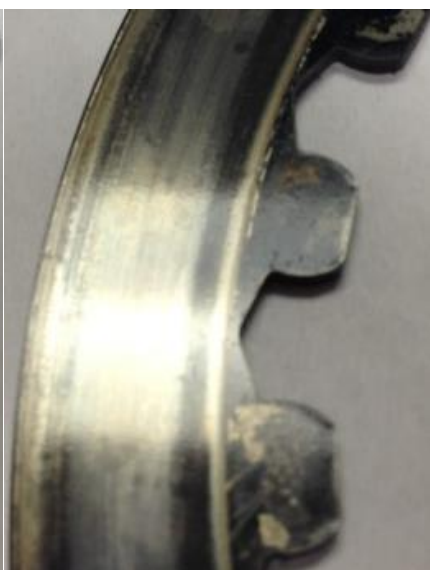
Excessive Heat (Black)
