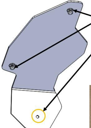
Remove Polaris Push rivets and install
