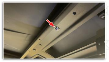
INSTALL THE M6X20MM SELF-TAPPING SCREWS AND 6MM WASHERS ON THE UNDERSIDE OF THE ROOF THROUGH THE FRAME ALONG THE FRONT OF THE VEHICLE.
