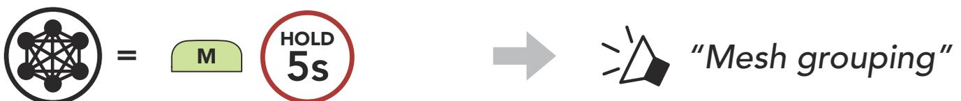
2. When **Mesh Grouping** is completed, the **users (You, B and C)** will hear a voice prompt on their headset as **Open Mesh** switches to **Group Mesh**.
