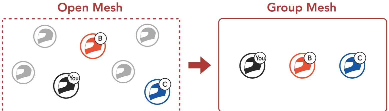
1. To enter **Mesh Grouping** to create a **Group Mesh**, press and hold the **Mesh Intercom Button** for **5 seconds** on the **users' (You, B, and C)** headsets.
