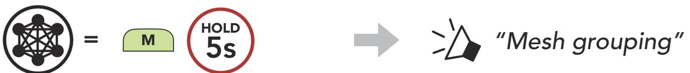
2. When **Mesh Grouping** is completed, the **new users (D and F)** will hear a voice prompt on their headset as **Open Mesh** switches to **Group Mesh**.
