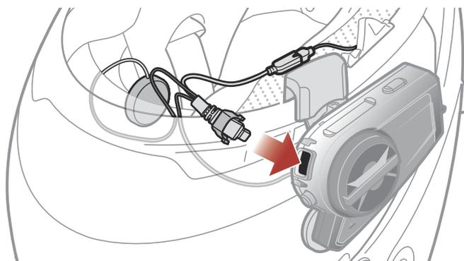
5. Close the cover of the speaker cable to lock the cable to the port.
