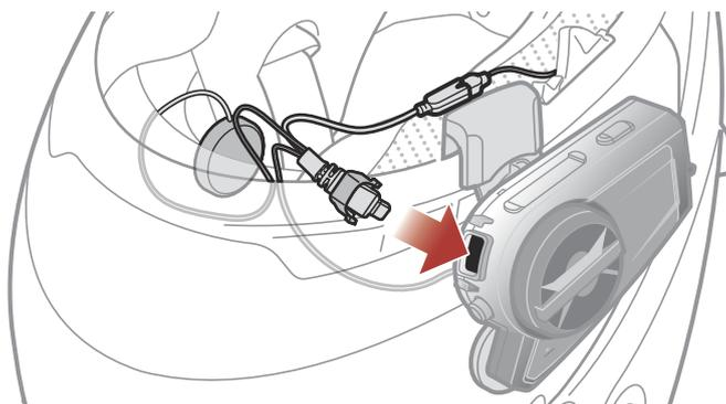
6. Close the cover of the speaker cable to lock the cable to the port.
