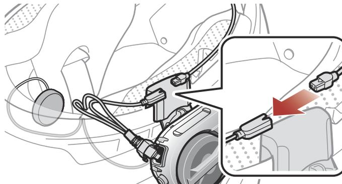
4. Insert the speaker cable into the speaker and microphone port to connect it to the main unit.
