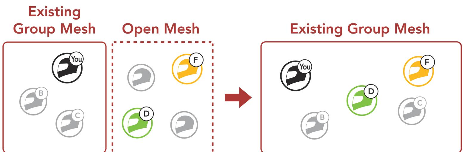
1. To enter **Mesh Grouping** to join the **Existing Group Mesh**, press and hold the **Mesh Intercom Button** for **5 seconds** on the headsets of **one (You) of the current users** in the **Existing Group Mesh** and the **new users (D and F)** in **Open Mesh**.
