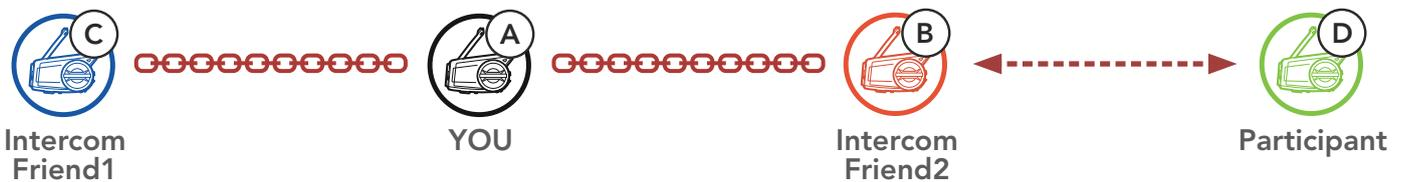
2. **Intercom friend (B)** can call a **new participant (D)** by tapping the **Jog Dial**, or a **new participant (D)** may join the intercom by making an intercom call to **Intercom friend (B)**.
