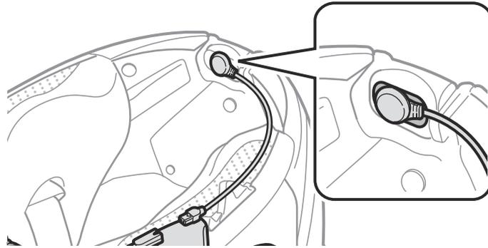
3. Align the arrows on the microphone and speaker cables and insert the microphone cable into the microphone connector.
