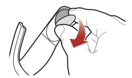
2. Insert the visor into the hole indicated in the illustration below.
