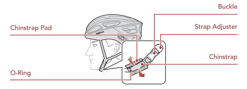
5. Secure the excess strap with O-ring and then attach the chinstrap pad. Always wear the helmet with the chinstrap buckle fastened and the chinstrap pulled tight and positioned back against the throat. With the strap buckled and the helmet positioned, you should feel the chinstrap pull firmly against your chin as you open your mouth. When properly adjusted the helmet will wrap around your head and cradle it with firm, but comfortable pressure.
