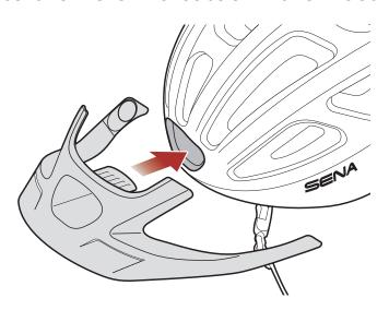
3. Align the hook and loop fasteners of the visor with the helmet and press hard to attach. Make sure that the visor sticks on the helmet firmly. Maximum adhesion occurs after 24 hours.
