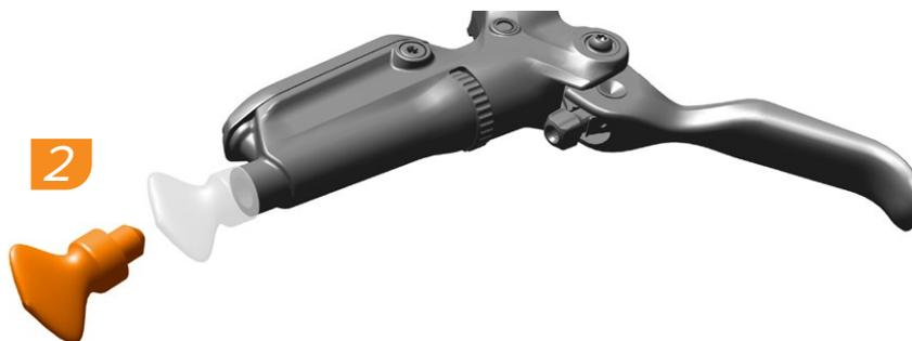
Remove the rubber lever body plug from the lever by pulling the plug straight from the lever. **Do not rotate the rubber lever body plug while removing.**
