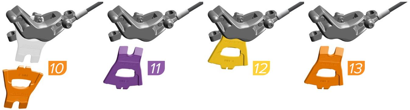
Remove the pad spacer from the caliper (10), rotate it 180 degrees (11), reinstall the pad spacer in the caliper (12), then remove the pad spacer (13).
