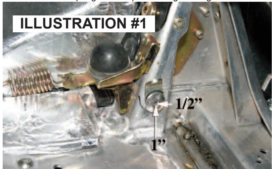
6. Using the small packet supplied, apply anti-seize to the threads of the exhaust temperature probe and re-install, torquing to 12 - 15 ft/lbs. It is very important to use anti-seize and the proper torque specification on the probe. Failure to follow these guidelines can cause damage to the probe during installation.
