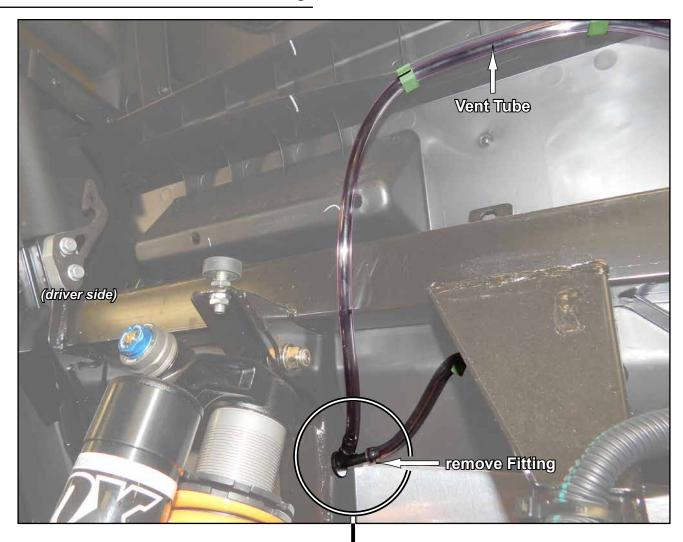
Rear Bracket contains mounting location for stock Vent Tube Mounting.
