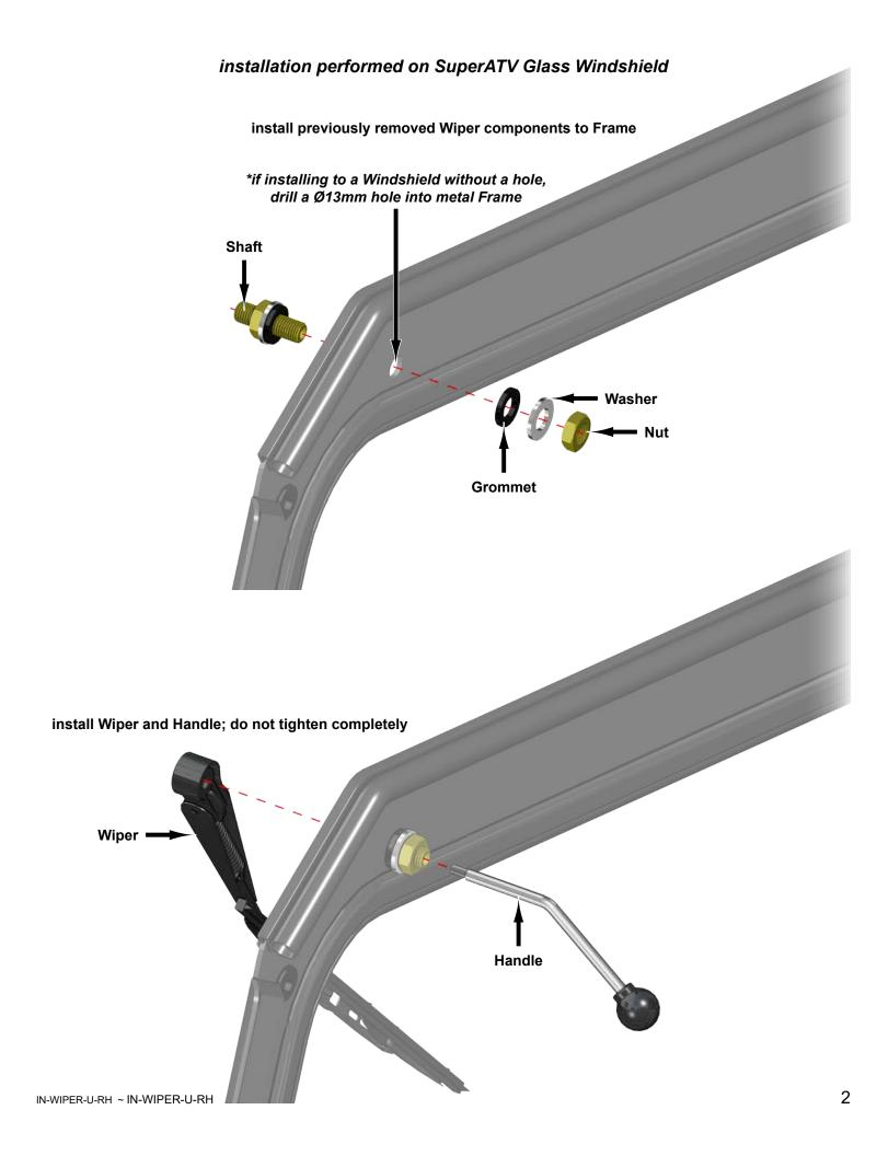
SuperATV recommends positioning Handle and Wiper as shown; tighten completely
