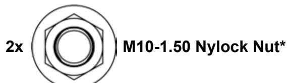
\*Use only if SuperATV Frame Stiffener is installed.
