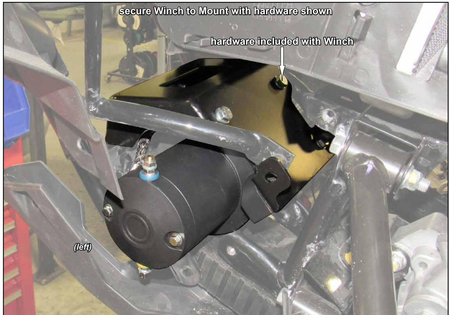
*tighten hardware completely*
