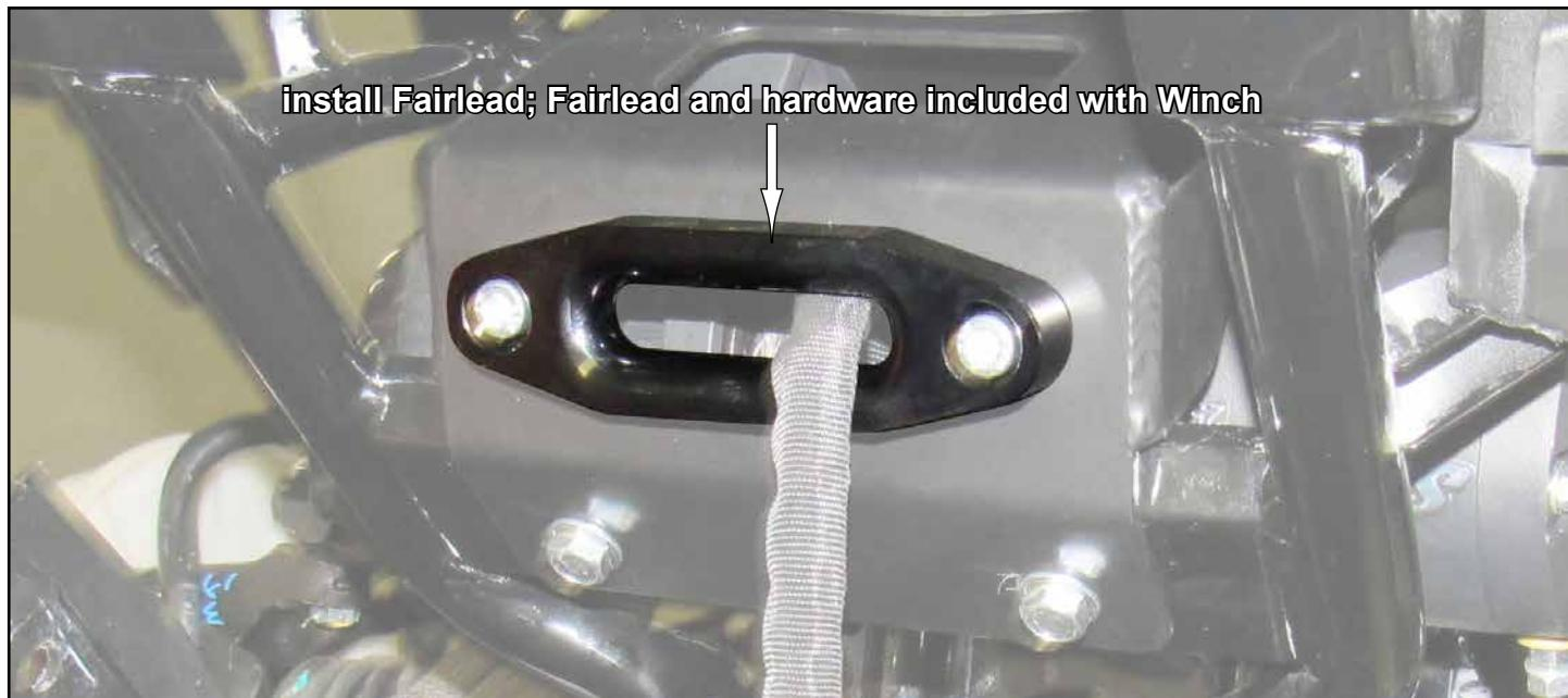
*tighten hardware completely*
