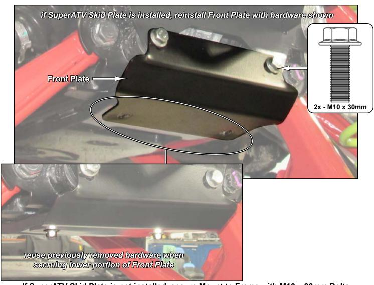
If SuperATV Skid Plate is not installed, secure Mount to Frame with M10 x 30mm Bolts.
