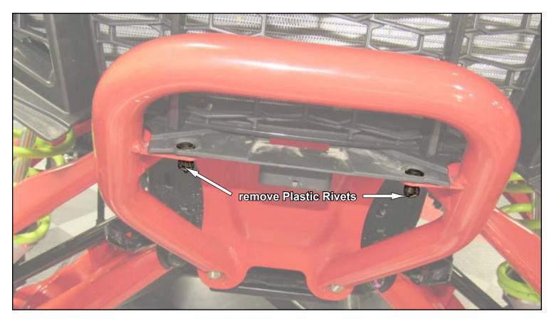
Remove Bumper and (4) Bolts. Bumper will not be re-installed.
