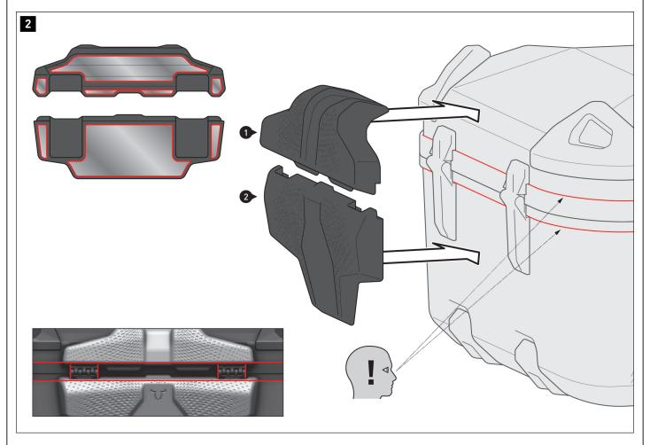
⚠ NOTE: Before re-installing, determine the position of the passenger backrests (1/2) on the lid and body of your DUSC. Make sure that the DUSC passenger backrests (1/2) rest on the frame profiles (marked in red; see illustrations below left and right).
