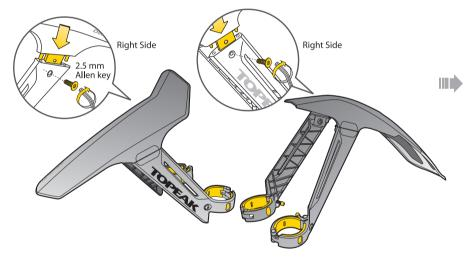
2. Loosen tension bolt on four fender legs.
