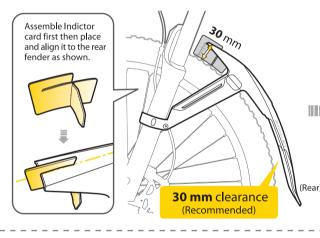
4. Make sure the rear fender is aligned with tire. Tighten both tension bolts and remove the Indicator Card.
