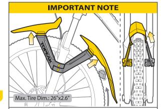
A unique design allows front fender to disengage due to any large obstructions entering the wheel.
