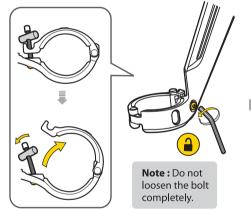
3. Install the rear fender to the fork legs and DO NOT tighten the tension bolts completely. Place the Indicator Card to the fender and adjust fender to make sure there is at least 30 mm clearance between fender and tire as shown.
