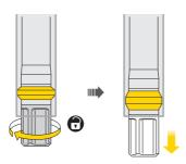
Turn Locking Grip clockwise to loosen the Rubber Ring and remove the pump.
