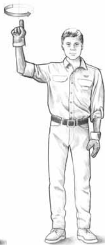
2) Power in the wire rope Hold your forefinger in the air above your shoulder height and draw small circles in the air to indicate to wind the winch.
