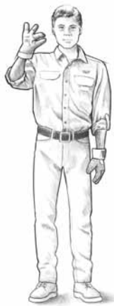
4) Pulse wind the wire rope Tells the driver to wind the winch in short, quick bursts. Open and close the two fingertips until you want the winch to stop.
