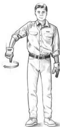
3) Power out the wire rope Hold your forefinger pointing down and draw circles in the air at about waist height to indicate feeding more wire from the winch.
