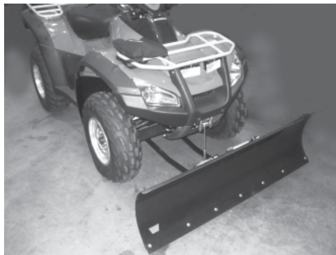
Figure 8 Completed Winch and Plow Assembly
