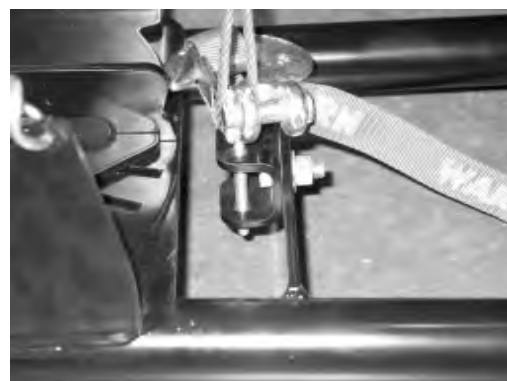
Figure 3 - J-Bolt Bracket and Winch
