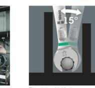
The Joker 6003 ring spanner with its special mouth geometry mouth side pivoted by 7.5° and the double hexagon profile doubles the placement possibilities when repeatedly turning the wrench 180° around the longitudinal axis. Bolts and screw heads can be "accessed" every 15°. The Joker 6003 will automatically find the respective placement point after every turn.
