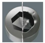
Hexagon socket screws are a problem, because the contact surfaces that transfer the force of the tool to the screw are very narrow. The consequence: the head of the screw can be damaged, usually rounding out the recess. Hex-Plus tools have larger contact surfaces to prevent this, driving from the flats of the recess, rather than the corners. Good to know: Hex-Plus tools fit into every standard hexagon socket screw!
