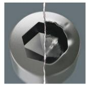
Hexagon screws can endure a problem because the contact surfaces delivering the power from the conventional tool, is transferred to the screw via very small surface areas. The consequence: the screw become damaged (rounding out). Hex-Plus tools have a greater contact surface that prevents this from happening! At the same time, as much as 20 % more torque can be applied. Good to know: Hex-Plus tools fit into every standard hexagon socket screw!
