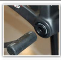
2. Start inserting adapters into bottom bracket bearings by hand. Seat adapters using a rubber mallet.
