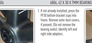
1. If not already installed, press the PF30 bottom bracket cups into frame. Remove outer dust covers. if present. (Do not remove the bearing seals). Identify left and right side adapters.
