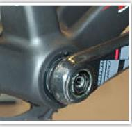
4. Take up any play in your cranks with supplied Crank Spindle Spacers. Place the spacers as needed.
