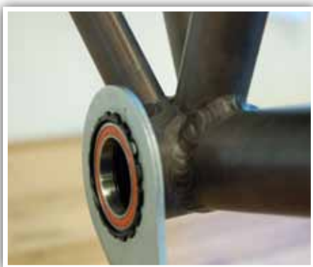
4. Use 16-notch BB tool - 48.5mm OD to thread drive side cup into frame until flush. Using torque wrench, fully tighten to 35-50Nm.
