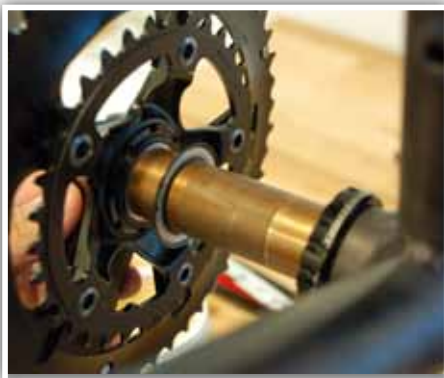
7. Install right crank arm, making sure outer dust seal is installed.
