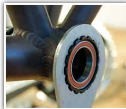
6. Use 16-notch BB tool - 48.5mm OD to thread non-drive side cup into frame until flush. Using torque wrench, fully tighten to 35-50Nm.
