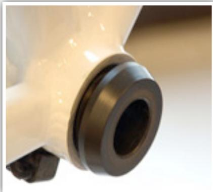
1. Confirm that all clips and bearings are installed into BB30 bottom bracket shell. Identify left and right side adapters and start inserting the adapters into the bottom bracket by hand.
