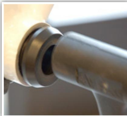
2. Seat adapters using a rubber mallet.
