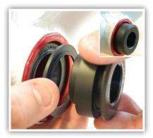
2. Insert the left side adapter with (1) 10mm spacer and (1) 5mm spacer. Left side spacers (30mm I.D.) fit between the left side (22mm I.D.) adapter and the BB shell. Spacers can be placed on either side to center cranks in bottom bracket.
