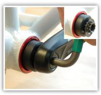
3. Install the crank. If there is side-to-side play, you may need 24 mm spacer(s) on the right side and/ or additional 30 mm spacer(s) inserted on the left side adapter. Tighten to manufacturer's specification. Crank should spin freely.
