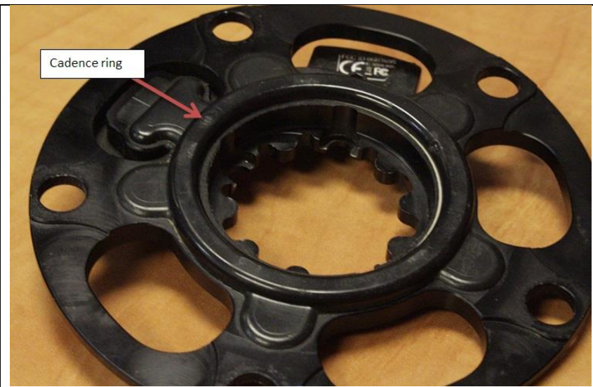
Older Quarq power meter. Note the protruding cadence ring. This power meter will not work with any Wheels Mfg bottom brackets that have 48.5mm x 16 notch cups.
