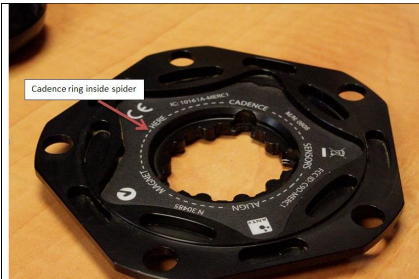
Quarq Riken power meter. Note the flatter cadence sensor ring. This powermeter is compatible with Wheels Mfg BBRight and BSA30 bottom brackets, but not with 386EVO, BB86/92 thread together, and T47 with inboard bearings when used in a 86.5mm wide shell.
