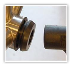
2. Seat adapters using a rubber mallet.
