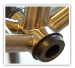
If not already installed, press the PF30 bottom bracket cups into frame. Remove outer dust covers, if present. (Do not remove the bearing seals). Start inserting adapters into bottom bracket bearings by hand.
