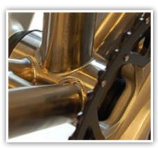
3. Install crank spindle through adapters and tighten per manufacturer's instructions. Take up any play in your cranks with our Crank Spindle Spacers and place as shown above.
