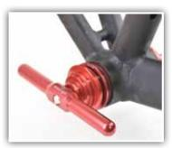
Insert drive side bottom bracket cup (female) in frame. Insert drift into bottom bracket bearing. Match up the correct size step on the drift with the bearing inner diameter.
