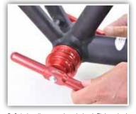
Spin handles onto threaded rod. Tighten both handles together until cup is fully pressed in frame.
