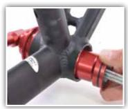
6. Insert the opposite bottom bracket cup in frame, leaving the drift and handle in the bottom bracket cup previously pressed in.
