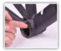
Thoroughly clean frame's bottom bracket shell. Do not install cups dry. Apply a thin layer of high quality grease, carbon-safe grease or anti-seize compound to inside surface of the frame's shell. Use the appropriate compound for your frame's BB shell material.
