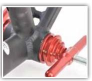
Insert second drift in bottom bracket bearing. Match up the correct size step on the drift with the bearing inner diameter. Spin handle onto threaded rod.
