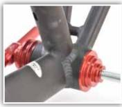
4. Insert other drift into the opposite side of the bottom bracket shell. Match up the correct step size with the shell diameter. Drift should fit with little to no play.
