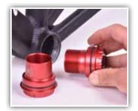
Lubricate each bottom bracket cup outer surface. Apply grease only to the cup threads.
