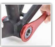
7. Using the BB wrench (<u>WRENCH-BB48-44</u>), fully tighten cup. Approximate torque 35-50Nm.
