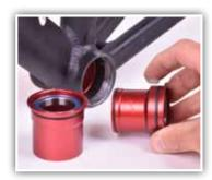
2. Lubricate each bottom bracket cup outer surface.
