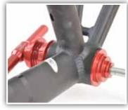
Insert other drift into the opposite side of the bottom bracket shell. Match up the correct step size with the shell diameter. Drift should fit with little to no play.
