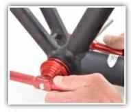
5. Tighten both handles together until cup is fully pressed in frame.
