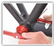
8. Tighten both handles together until second cup is fully pressed in frame.
