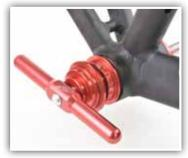
3. Insert drive side bottom bracket cup in frame. (If installing BBRIGHT-OUT, install non-drive side cup.) Insert drift into bottom bracket bearing. Match up the correct size step on the drift with the bearing inner diameter.
