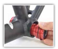
Insert opposite cup into frame by hand until threads begin to engage. Pay careful attention to not cross-thread cups. Turn in BB cup aas far as possible by hand.
