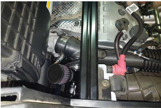
14. Adjust components to provide a satisfactory fit. Maintain a minimum of ½" clearance around parts, while allowing for vibration.
