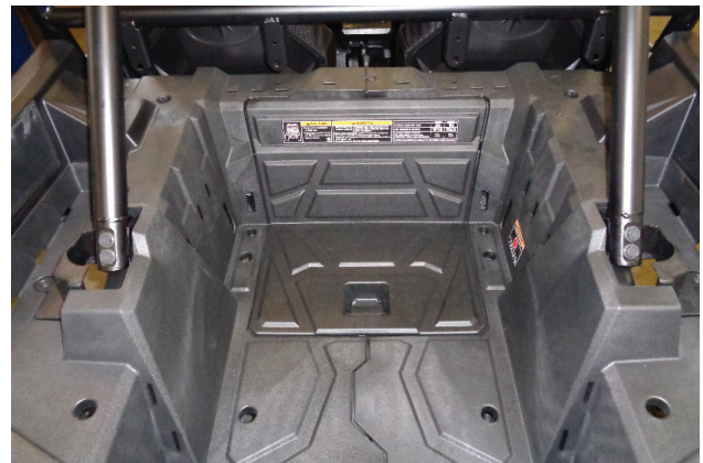
16. Replace cover on air box compartment.
