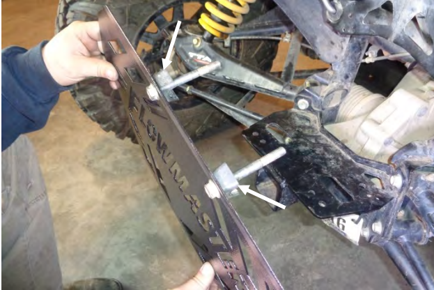
11. Assemble the bolts and fascia clips to the holes at the top of the heat shield (5).
