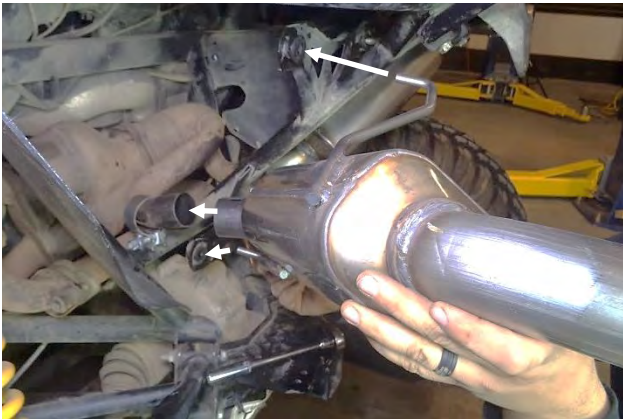
7. Grease the two mount rods on each muffler. Install each muffler (3, left; and 11, right) onto its exhaust pipe, while pushing its two mount rods into their rubber hangers.
