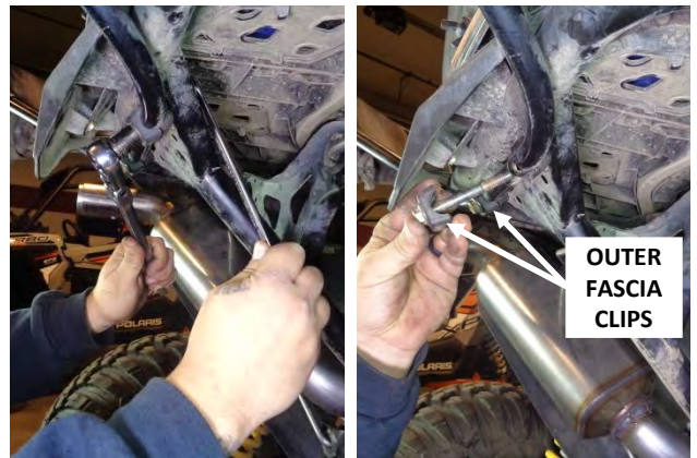
10. At the middle of the tail-light support tube (behind the "BPR" medallion), remove the two bolts and nuts, and only the two outer fascia clips (that is, just the clips under the bolt heads).
