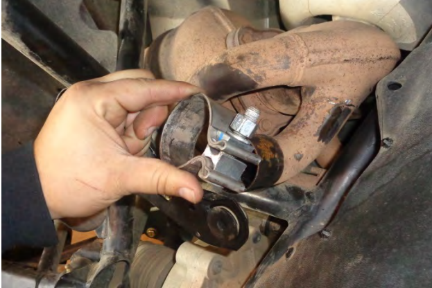
6. Slip a clamp over each exhaust pipe.
