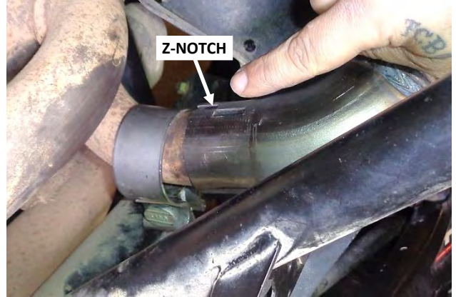
8. Note the locations of the two Z-notches (180° apart) on each muffler inlet.
