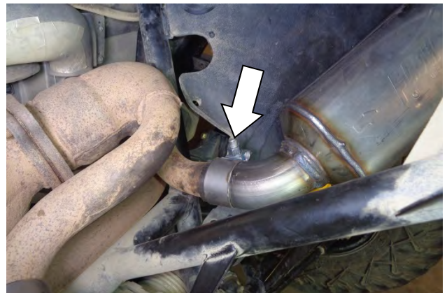
9. Align the clamp so that its gap is NOT aligned with either Z-notch (that is, the clamp band covers both Z-notches), then tighten the clamp.
