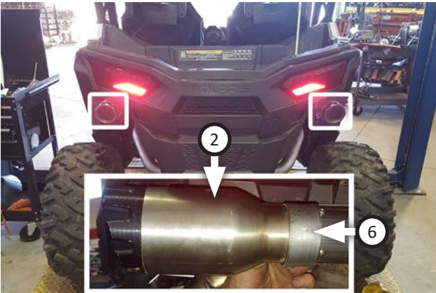
13. Place 2 clamps (6) onto exhaust tips (2) , then connect them to tailpipes. Tighten clamps to secure connection.
