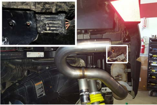
12. Re-connect rear taillight harness as shown.
