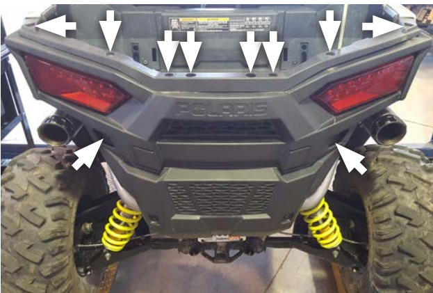
14. Install remaining 10 screws (removed step 2) to complete fascia install.
