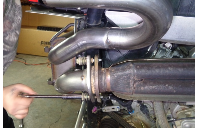
22. Apply anti-seize compound to the two flange bolts, install them, and tighten them down evenly.
