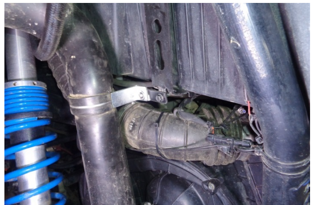
18. Secure the bracket to the vehicle using the stock clamp bolt, adjusting the position of the duct as required.
