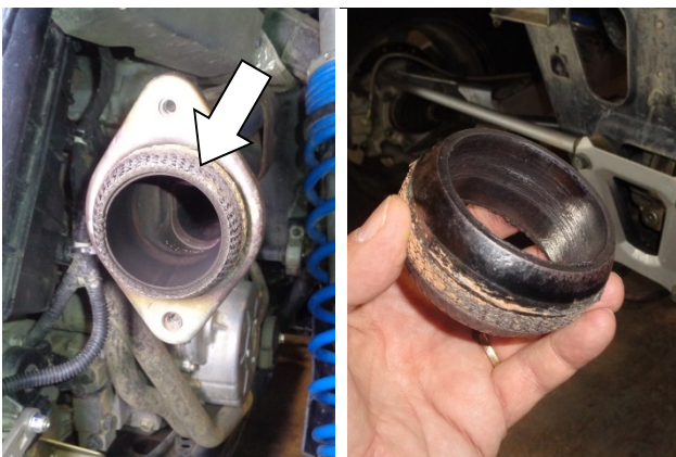
15. Inspect the lead gasket on the end of the exhaust pipe for serviceability. Replace if required.
