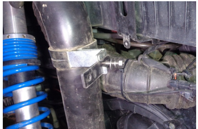
17. Assemble the bracket (item 11) to the clamp, using the 1/4-20 screw (6) (on the outboard side), 2 flat washers (7) (one on each side), and the lock washer (9) and nut (10) (on the inboard side).
