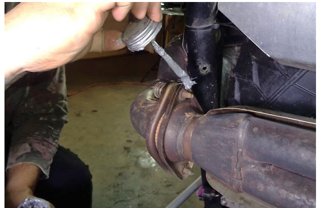
11. To prevent seizing of the flange bolts during removal, apply penetrating oil or anti-seize compound to the exposed threads.
