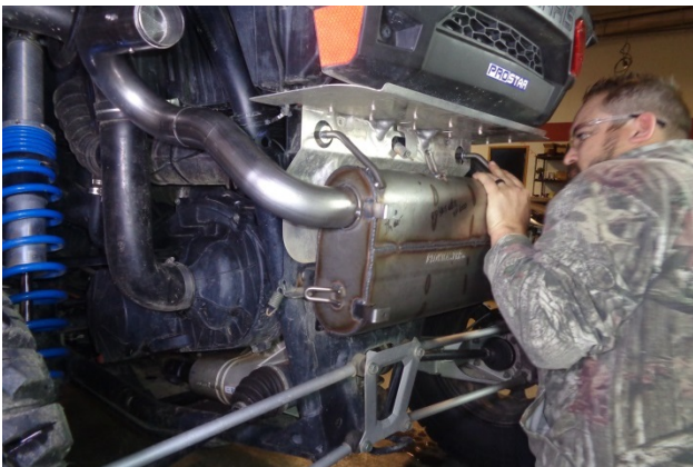
20. Install the new muffler (1) by pushing the two hanger pins into the rubber mounts. Ensure proper alignment the exhaust pipe and muffler flange.
