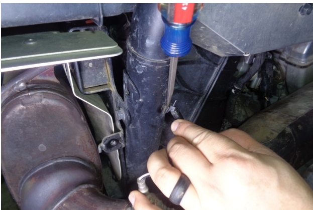
9. Carefully remove the O 2 sensor lead clamp from the vehicle frame.
