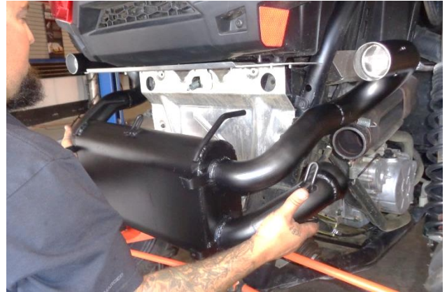
10. Install the new muffler (item 1) by pushing the two hanger pins into the rubber mounts. Ensure proper alignment the exhaust pipe and muffler flange.
