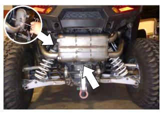
9. Use a spring puller to connect the two muffler mount springs to the new muffler.
