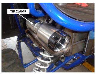
1. Loosen the exhaust pipe tip clamp and remove the tip.
