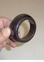
7. Inspect the lead gasket on the end of the exhaust pipe for serviceability. Replace if required.
