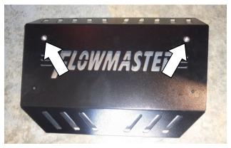
12. Place the heat shield (4) over the spacers and place flat washers (7) over the top two holes. Align the backer, spacer and the shield holes, and insert screws (6) in them.
