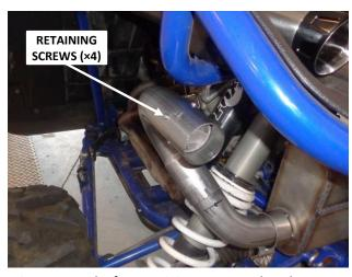
2. Remove the four retaining screws and washers.
