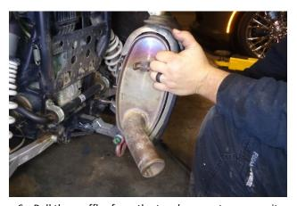
6. Pull the muffler from the two hangers to remove it from the vehicle.
