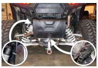
5. Use a spring puller to release the two muffler mount springs.
