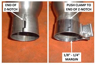
17. With that note in mind, install a clamp on each exhaust tip (3). For best retention, push the clamp just to the end of the Z-notch, leaving 1/8" to 1/4" of the clamp extending past the tip opening.
