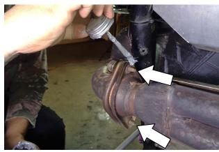
3. To prevent seizing of the exhaust flange bolts during removal, apply penetrating oil or anti-seize compound to the exposed threads.
