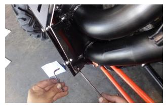
15. After the nuts have been started on all 4 screws, tighten the fasteners.
