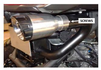
18. Push each tip onto its pipe until its clamp touches the spark arrestor screws. Orient the clamp bolts inboard and the nuts down (per Step 16). Also, keep the rear edge of the clamp just over the end of the Z-notch (per Step 17). When each tip is in place, tighten its clamp.
