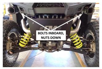
16. Note that the bolts on both tip clamps (2) will be oriented inboard, with the nuts pointed down.
