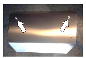
11. Place the heat shield backer (5) on a bench or other flat surface. Place spacers (8) over the top two holes.
