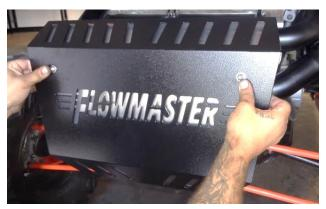
13. Grasp the aligned heat shield, backer and hardware and hang the assembly on the muffler's two top mount holes. Then install a flat washer (7) and lock washer (9), and hand-start a nut (10), on each screw.
