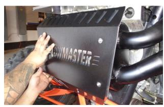
14. At each bottom hole, hold a spacer (8) in between the heat shield and backer. Install a screw (6) with flat washer (7) through the stacked parts. Then install a flat washer (7), lock washer (9), and nut (10) on each screw.
