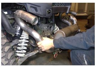
Install the new muffler (item 1) by pushing the two hanger rods into the rubber mounts. Ensure proper alignment of the exhaust pipe and muffler flange.
