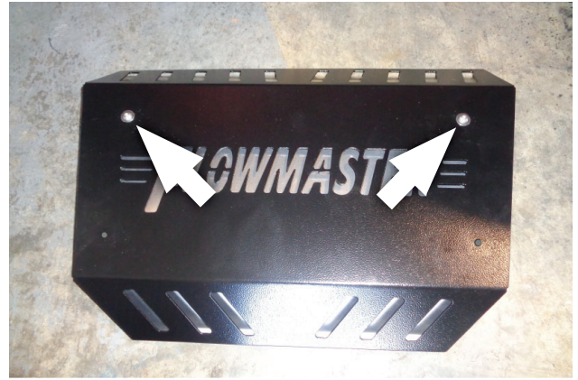
28. Carefully lay the heat shield (5) over the spacers, and place flat washers (7) over the top two holes. Align the backer, shield and hardware holes, and insert screws (6) in them.
