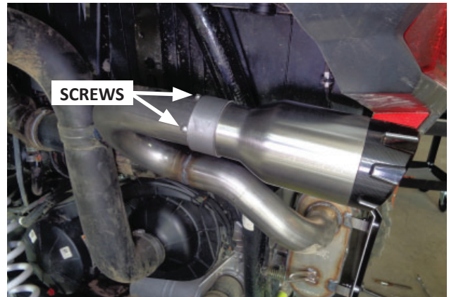
34. Push each tip onto its pipe until its clamp touches the spark arrester screws. Also be sure to keep the rear edge of the clamp just over the end of the Z-notch (per Step 32). When each tip is in place, tighten its clamp.
