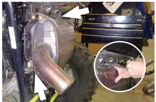
12. Use a spring puller to release the 2 muffler mount springs.
