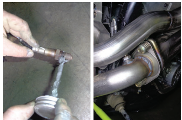
24. Apply anti-seize compound to the O2 sensor threads. (Do not get compound on the tip of the sensor.) Then install the sensor in the exhaust pipe.
