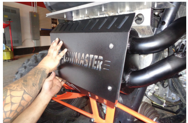
30. At each bottom hole, hold a spacer (8) in between the heat shield and backer. Install a screw (6) with flat washer (7) through the stacked parts. Then install a flat washer (7), lock washer (9), and nut (10) on each screw.
