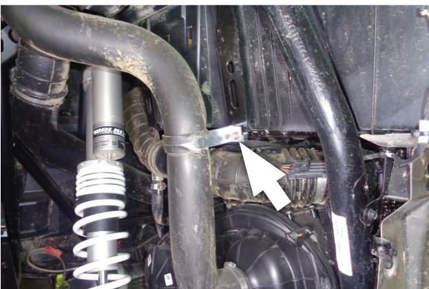
15. In the left rear wheel well, remove the bolt securing the clutch cooling air duct clamp to the frame.
