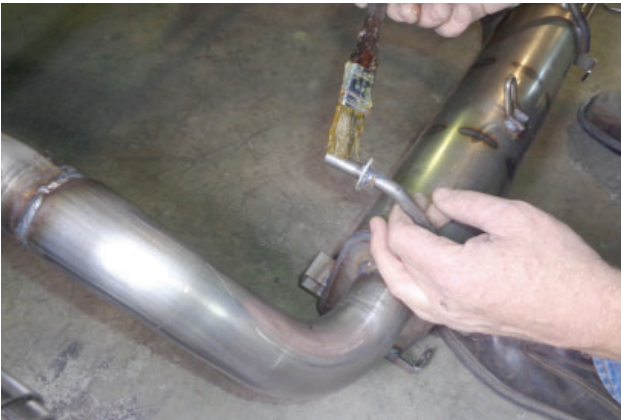
20. Lubricate the 2 hanger pins on the muffler (1) with grease or oil.
