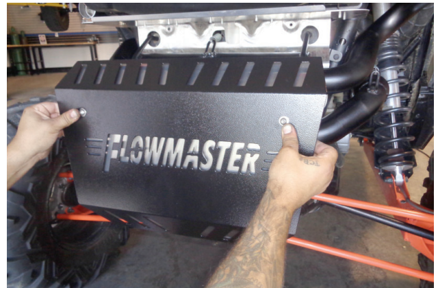
29. Grasp the aligned heat shield, backer and hardware, and hang the assembly on the muffler's two top mount holes. Then install a flat washer (7), lock washer (9), and nut (10) on each screw. NOTE: Do not tighten the nut at this time.
