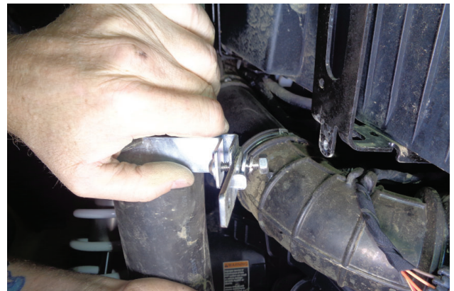
17. Assemble the bracket (item 11) to the clamp, using a screw (6) and flat washer (7) (on the outboard side), and a flat washer (7), lock washer (9) and nut (10) (on the inboard side).
