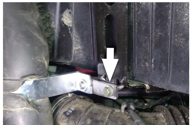
18. Adjust the alignment of the duct as required, and secure the bracket to the vehicle using the stock clamp bolt.
