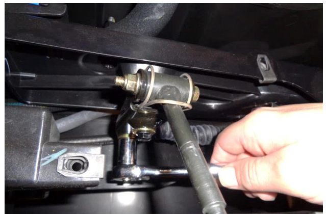
19. Remove the nut and washer connecting the shift lever to the cable. (Only the nut will be reused at Step 32 .)
