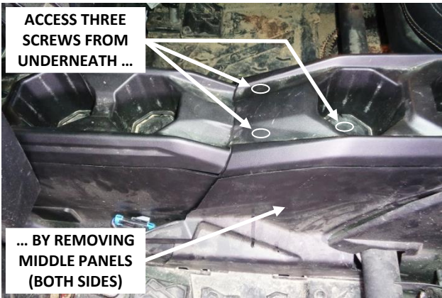
9. Gain access to the 3 screws securing the front of the middle console cover as follows ( Steps 10-13 ).
