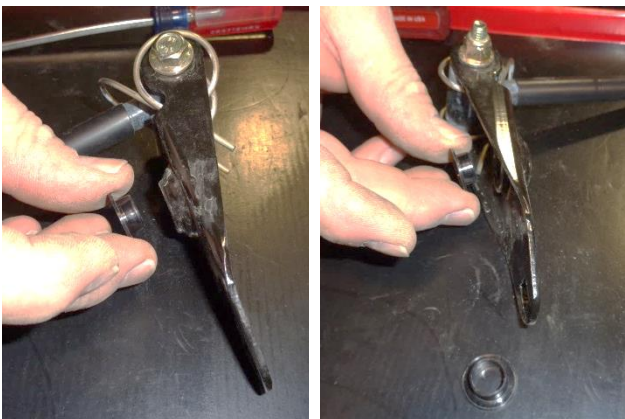
22. Remove 2 plastic sleeves from shifter for use at Step 30.
