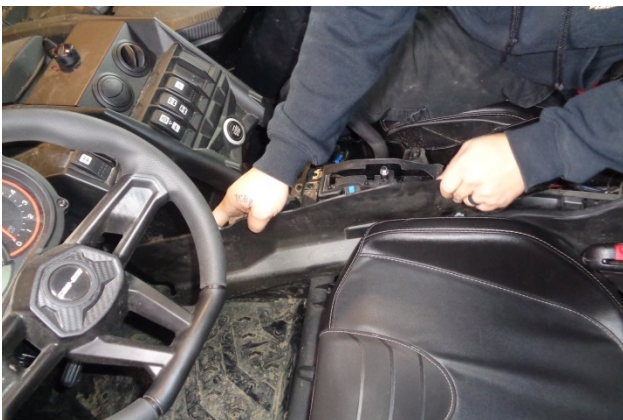
16. Remove both front side panels.
