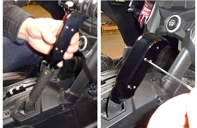
53. Slip the passenger grab handle onto the tube, align it as desired, and tighten the 8 set screws.
