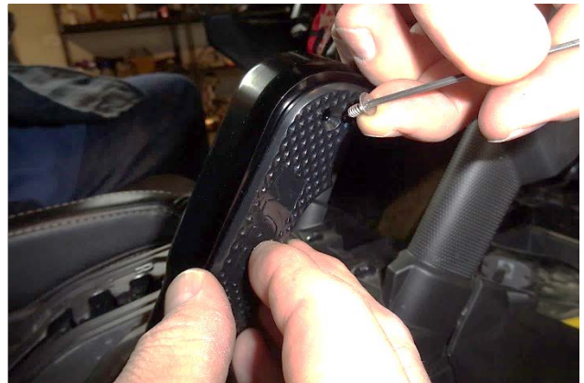
54. Reinstall the grab handle side plates.
