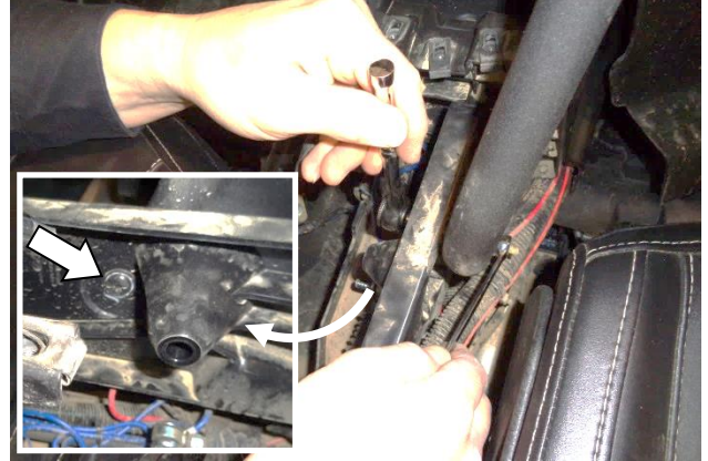
23. Remove the screw, nut and washer securing the grab handle tube to the frame. (Only the screw and nut will be reused at Step 36. )
