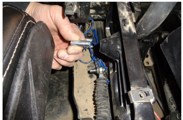
31. Install the pivot bushing in the pivot bore in the frame.
