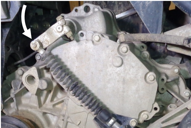
57. Manually verify that the shift arm is rotated fully forward.
