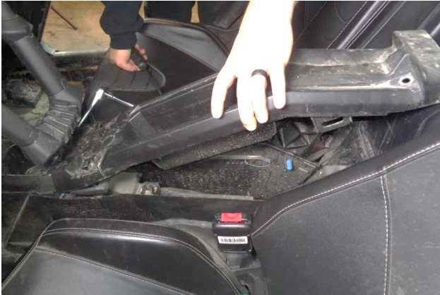
8. Remove rear console cover.
