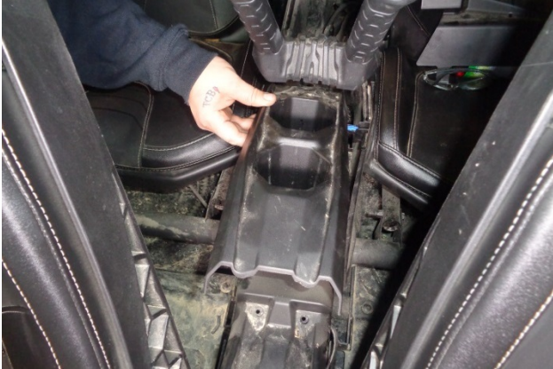
14. Remove middle console cover.
