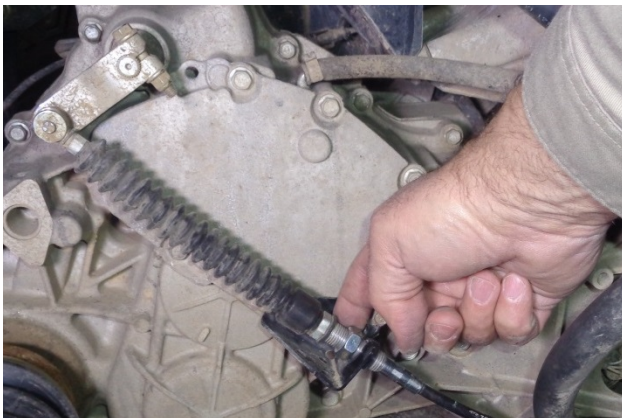
58. Turn both nuts back by hand until they are equally snug against the cable bracket.
