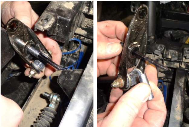
21. Remove the pivot bushing for use at Step 31.
