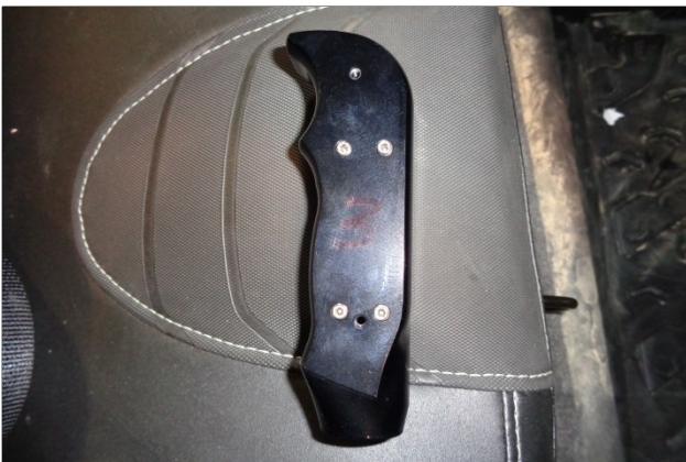
52. Remove the two side plates from the passenger grab handle assembly (2), then back out the 8 set screws sufficiently to permit the handle to fully slide onto the handle frame.
