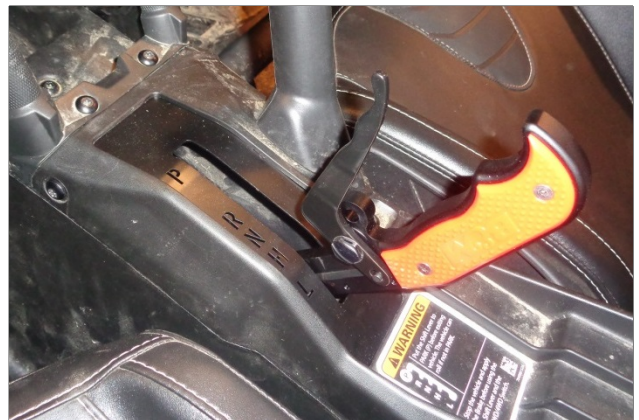
55. Lock the shift handle in LOW.
