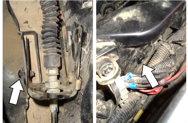
29. Reinstall the cable support in the frame. Hand-start (do not tighten) only the 2 rear screws. (The other 2 screws will be used at Step 35. )
