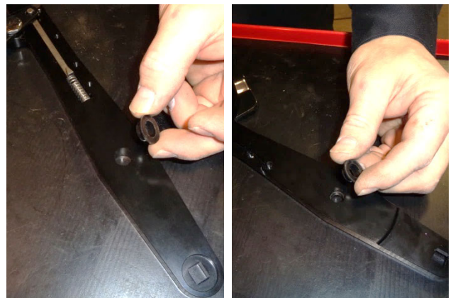
30. Install the 2 plastic sleeves in the shift lever assembly (3).
