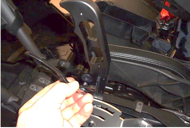
38. Remove the shoulder bolt, locking lever and spring washer. NOTE: Do not lose the spring washer (located under the bolt head).
