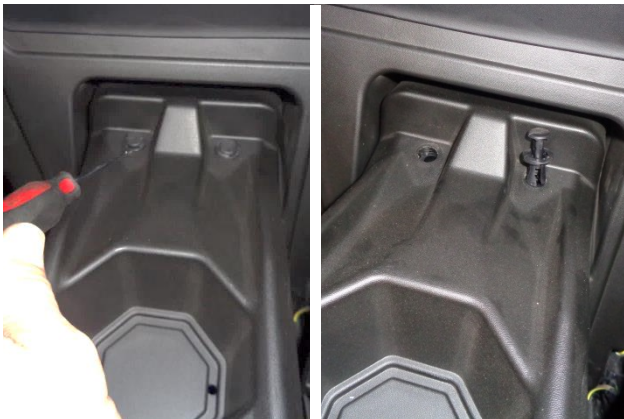
51. Secure rear of the console cover with its 2 plastic push rivets.
