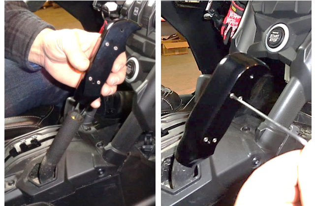
53. Slip the passenger grab handle onto the tube, align it as desired, and tighten the 8 set screws.
