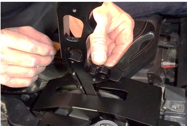
40. Reinstall the locking lever, spring washer and bolt. Ensure that the lever's short leg properly engages the selector pin.
