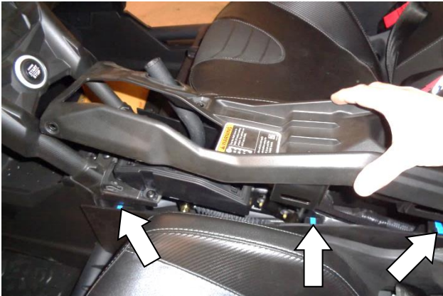
15. Carefully unsnap the 3 clips on each front side panels. Then remove front console cover.
