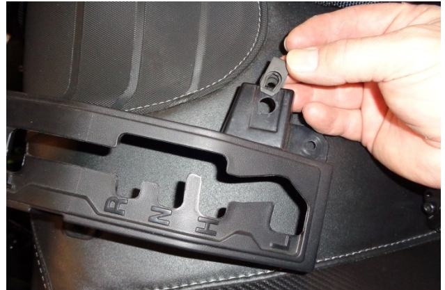
18. Remove the nut plate from right side of the shifter gate for use at Step 39 .
