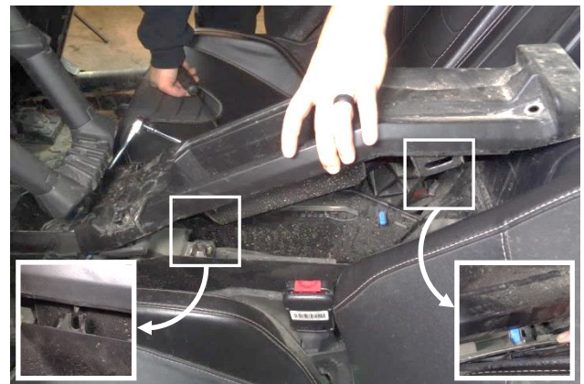
49. Install the rear console cover, aligning pins with their notches, and snapping the clips into their slots.
