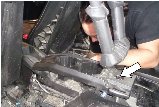
44. Put the middle console cover in place, and hand-start (do not tighten) the rear screw.
