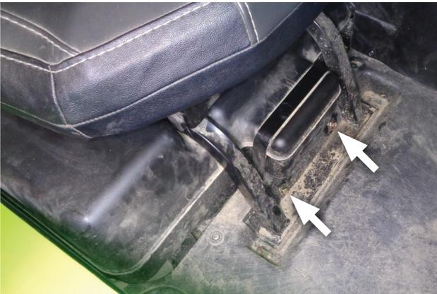
38. Re-install screws (x2) (removed step 4) to secure base of passenger seat to frame.
