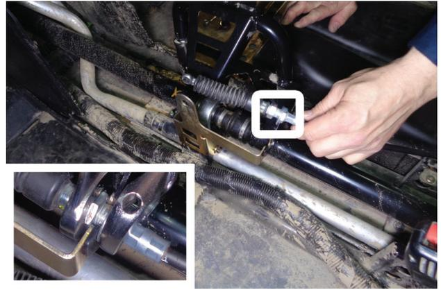
16. Loosen nuts in order to remove shift cable from support bracket.
