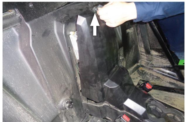
6. Remove rear console cover from vehicle. Retain for later use.
