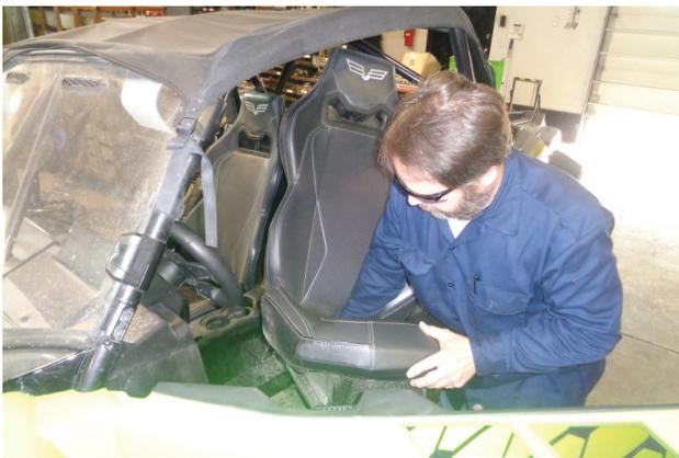
3. Release locking mechanism and remove driver seat from vehicle as shown.
