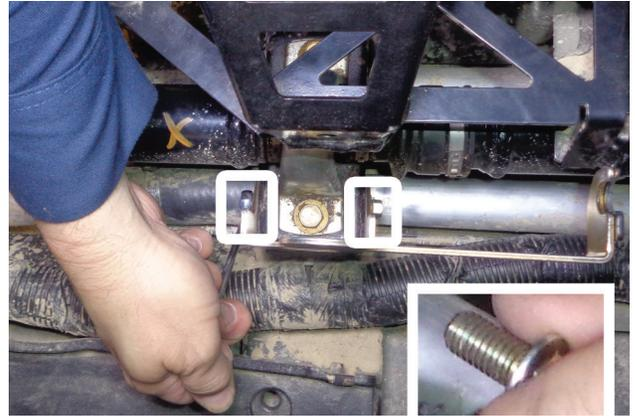
17. Remove cap screws (x2) securing support bracket. Retain for later use.
