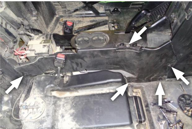
33. Install screws (x5) (removed step 10) to secure passenger side console cover to frame as shown.
