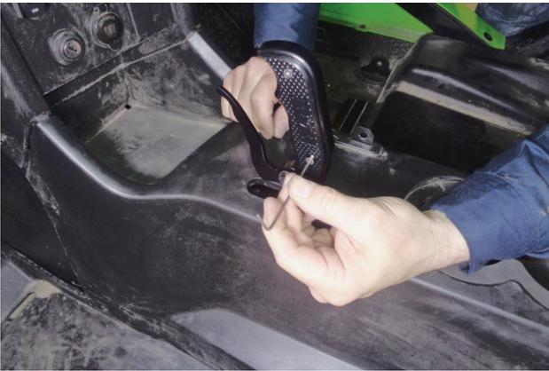
32. Install screws (x4), left shifter plate and right shifter plate back onto gated shifter stick (removed step 28).
