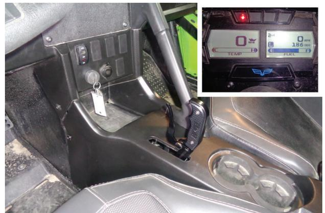
40. Move your shifter through all gears and make sure each one engages properly and is synchronized with the gear indicated on dashboard display.
