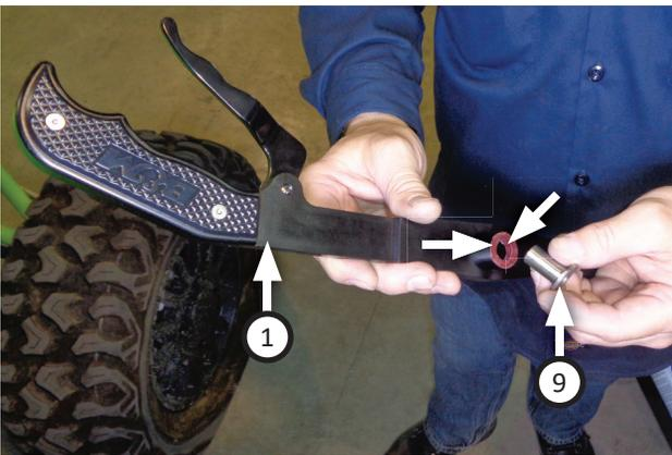
20. Install bushings (x2) from previous step onto both sides of **gated shifter stick (1)**. Install **spacer sleeve (9)** into passenger side of gated shifter stick.
