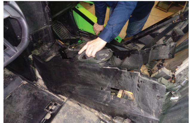
30. Fit console cover (removed step 12) over gated shifter stick into position as shown.
