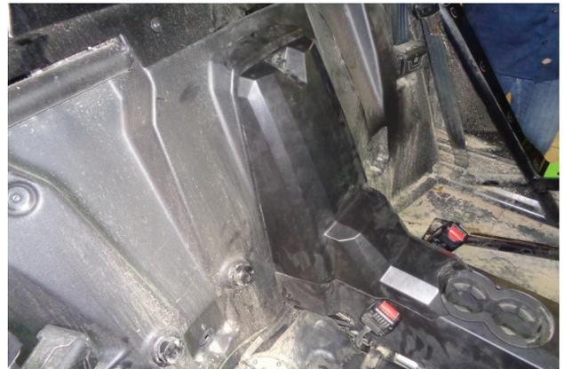
36. Re-install rear console cover (removed step 6) back onto console.
