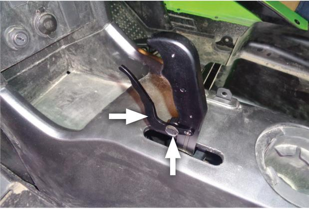
31. Install bolt, curved spring washer and lever onto gated shifter stick (removed step 29).
