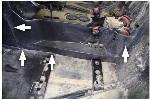
11. Remove screws (x4) securing driver side of console cover. Retain them for later use.
