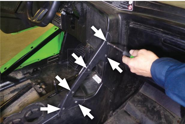
8. Remove screws (x6) securing handle to frame. Retain for later use.
