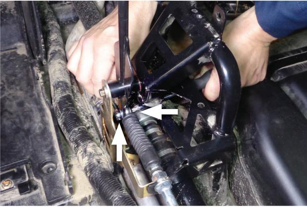
13. Remove factory shoulder screw and lock nut securing shift cable to lever.
