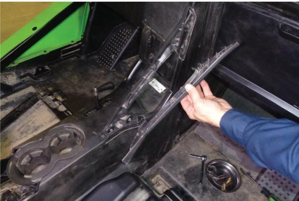
9. Remove left and right handle from console and dashboard. Retain for later use.
