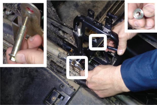
14. Loosen then remove factory shoulder screw and lock nut from shift lever.
