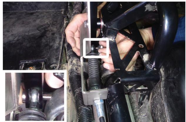
24. Place shift cable into gate plate while fitting its end into base of gated shifter stick. Secure shift cable to gated shifter stick using **screw (12)** on driver side through **lock nut (14)** on passenger side.
