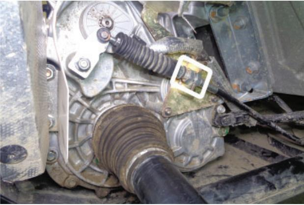
41. If shifter engages improperly, adjust shift cable nuts where indicated.
