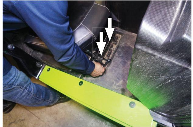
4. Remove screws (x2) securing base of passenger seat to frame. Retain them for later re-use.
