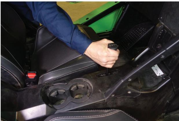
2. Turn off ignition, set shifter into neutral and securely chock vehicle's wheels to keep it from rolling.
