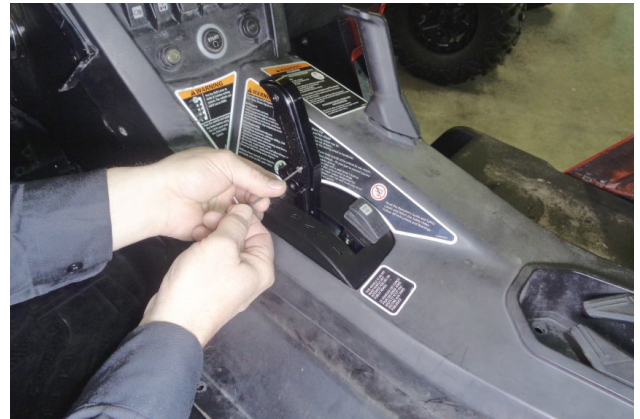
46. Install screws (x4) and grip shifter plates (x2) (removed step 21) onto shifter stick.
