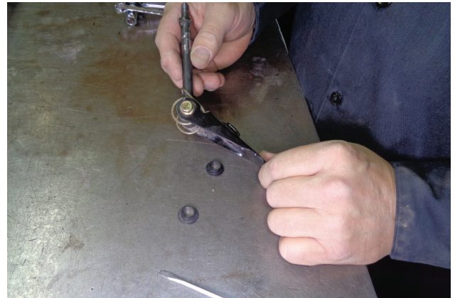
16. Remove metal sleeve and plastic bushings (x2) from shift lever. Retain bushings (x2) for later use.
