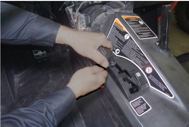
7. Shift vehicle into Reverse gear, then twist to remove factory shifter grip handle.
