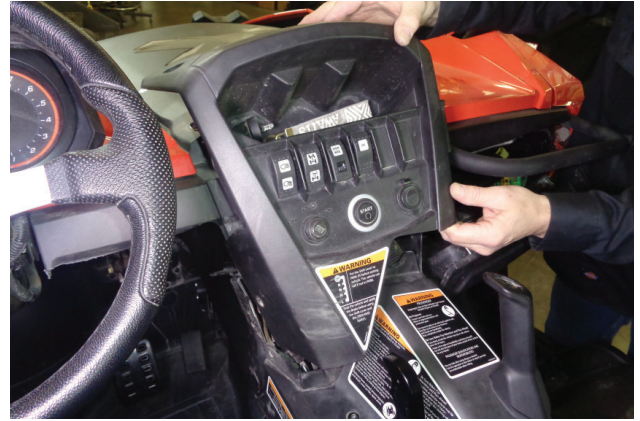
45. Install control panel (removed step 5) back in place onto dashboard. Install (x2 ea.) screws and push rivets (removed step 4) to fasten panel.
