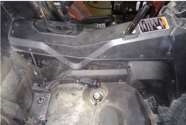
43. Fasten console top passenger side by installing push pins (x4) (removed step 9).
