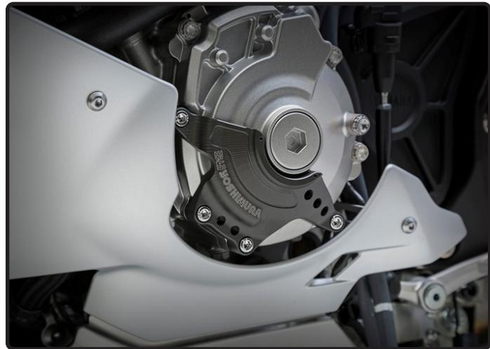
5. Install Yoshimura right side case saver using the supplied bolts. See diagram on page 1 for proper orientation and order of hardware.
