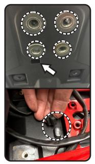
5. Route license plate light wires through loops on (No. 1) *19135-FEBKT*, fender eliminator bracket and through hole in undertail where the rubber cover was previously removed.
