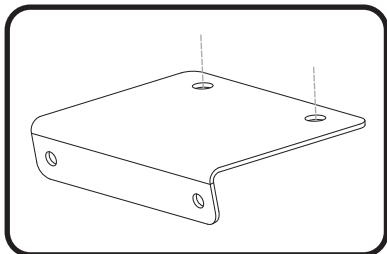
2. Install (No. 2) 12350-FEBKT-B, light bracket to (No. 1) 12350-FEBKT-A, fender eliminator bracket using (No. 10,11,12) 6mm bolt, washer, and lock nut.
