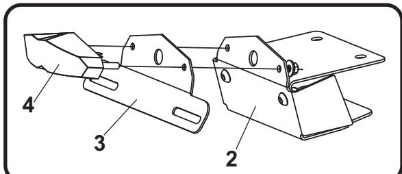
4. Install stock turn signals onto (No. 6,7) 12350-TSB-L/R, left and right turn signal brackets using the stock hardware.
