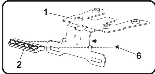
2. Install (No. 1) 12401-FEBKT, fender eliminator bracket using the four stock fender bolts and washers.
