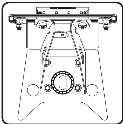
8. Re-connect license plate light and turn signal wires.
