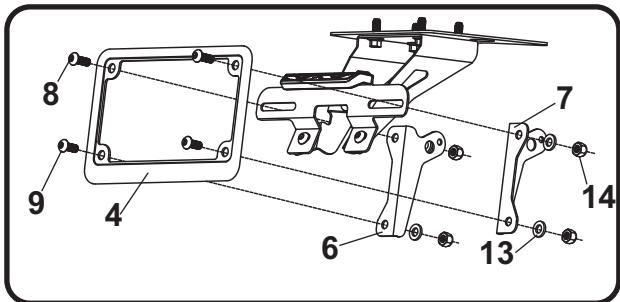
7. Route license plate light and turn signal wires through hole in bracket and through undertail.
