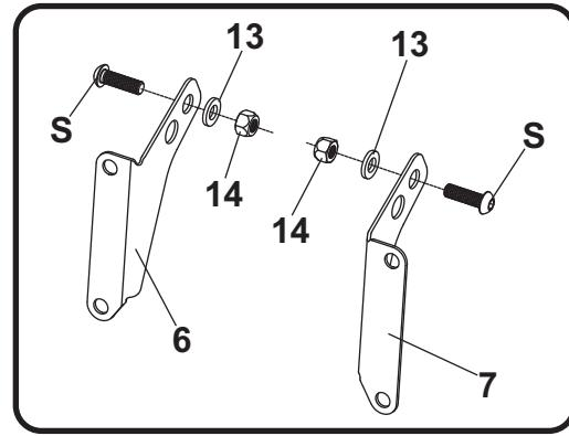
3. Install (No. 3) 12200-FEBKT, license plate bracket onto (No. 1) 19675-FEBKT, fender eliminator bracket using (No. 11) M6X10BHS, 6mm button head screw.
