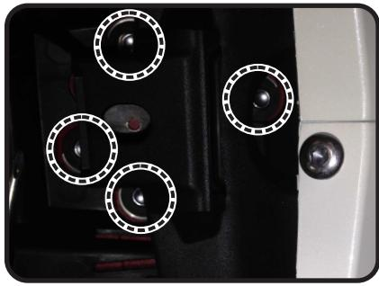
4. Remove the four fender mounting collars from subframe as they will not be used with the Yoshimura fender eliminator kit.
