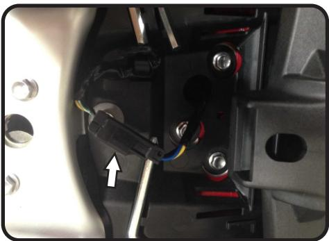
3. While securely supporting the stock fender assembly, remove the four bolts securing the fender assembly to the frame. Carefully remove the stock fender assembly making sure not to damage the connectors in the process.
