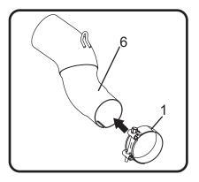
Install (No. 2) 03019135, exhaust clamp to (No.7) 11211-427, right tail pipe. **Do not torque at this time.**
