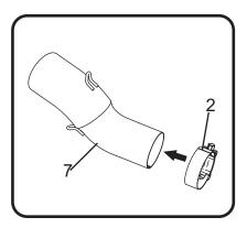
2. Install (No. 9) *HT SHLDR77*, muffler clamp heat shields to (No. 5) *1121-MPCRX*, muffler clamps and slide onto both mufflers.
